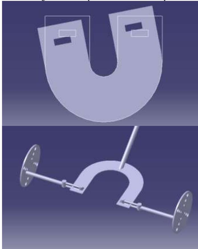
Fig.2. Rotation of Inverted U plate about fixed axis
