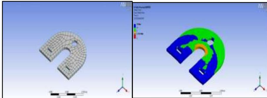
Fig.5 Meshed Modal of Horseshoe plate Fig.6 Fatigue Safety Factor
